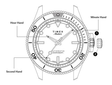
Pull out the crown to position **2**Turn until the desired time is reached, return the crown to position **1**
