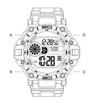
Button A: Reset/Stop Button B: Mode Button C: Lig ht/-Button D: Start/+
